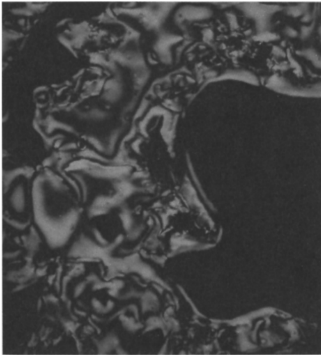
Figure 2. Optical micrograph between crossed polars at 185°C of the organometallic copolymer.
